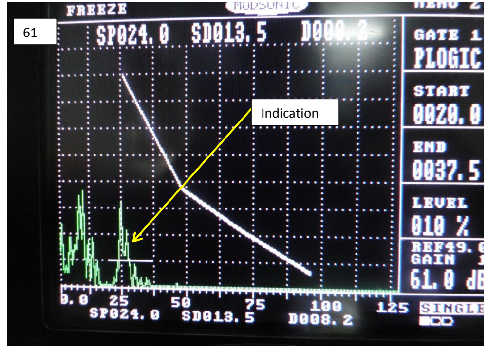
Cluster porosity response @ DAC (49db) + 12 db
