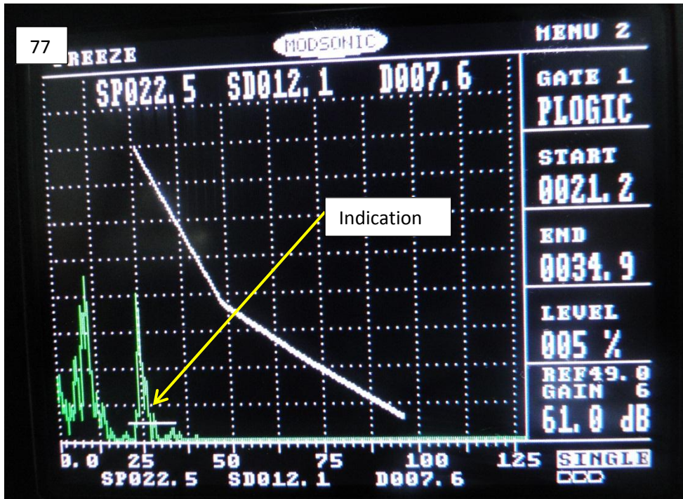
Center Crack response @ DAC (49db) + 12 db
