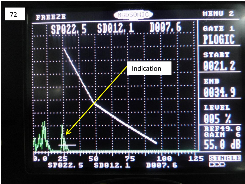
Center Crack response @ DAC (49db) + 6 db
