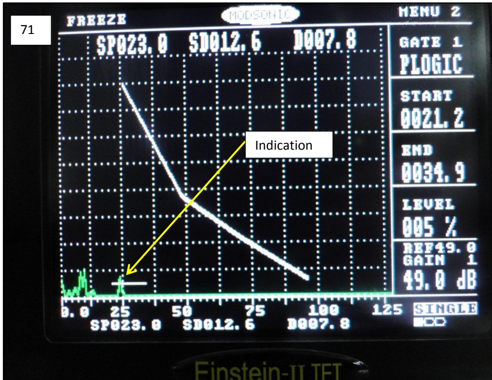
Center Crack response @ DAC (49db)
