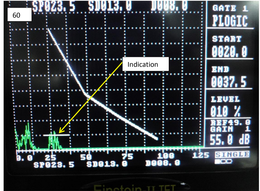
Cluster porosity response @ DAC (49db) + 6 db
