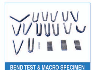
BEND TEST & MACRO SPECIMEN
